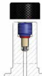
Model of valve stem integrated 5/8" 18 UNF (D)
